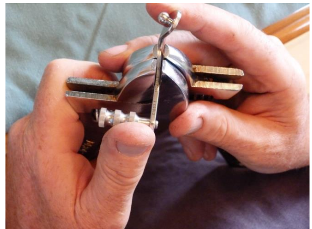
Figure 3-18 Stainless steel crescent wrenches (or bending irons) are used to accurately twist the femoral component without introducing any additional bend.
