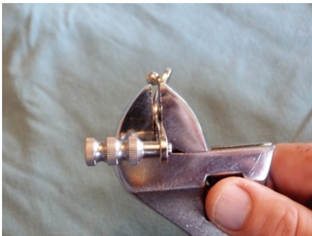
Figure 3-18 Stainless steel crescent wrenches (or bending irons) are used to accurately twist the femoral component without introducing any additional bend.
